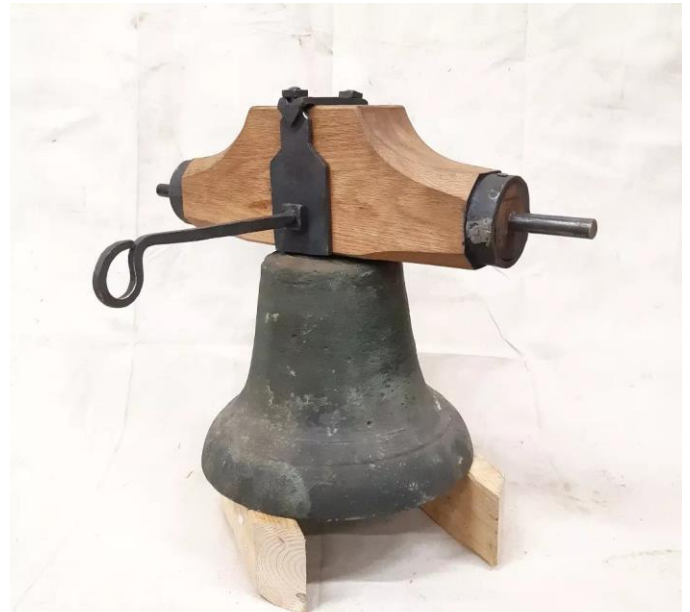
The bell, with a reconstructed yolk and new iron fittings made by Evan Meisner
